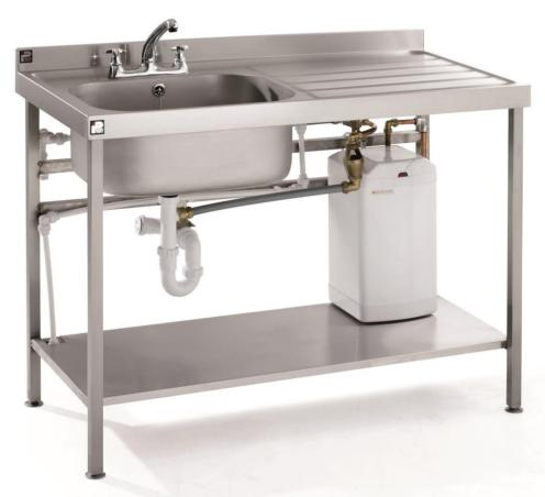
The Quick Fit Heated Sink is an innovative and flexible unit designed for ease of use in event catering or in permanent kitchens. The QFSINK uses a standard ¾ BSP connection and the supplied water heater works off a 13 amp plug, making the unit easy to install and disconnect.
